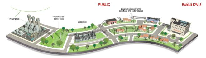
Power is generated at the plant and this could be a nuclear power plant, solar site, or wind farm. It is transmitted via the transmission power lines to the substation, where high voltage power is stepped down to a lower voltage. This lower voltage power is then distributed over distribution power lines to neighborhoods, businesses, and residences and ultimately into your homes.
